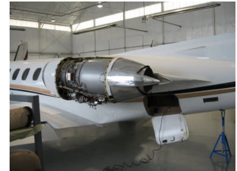
Citation II undergoing routine Phase B and calendar inspections.
