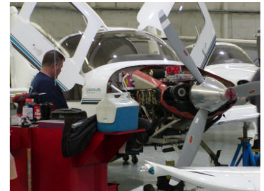
Scott Shaw, Lead Technician performing a Pre-buy/Annual inspection on a SR20 Cirrus N20CD.
