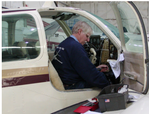
Jack Musgrave, Avionics Manager installing a Garmin GMA 340 Audio Panel in a Beech Baron N43BS.
